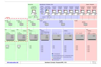
The interfaces between the controllers and the connection of the periphery are made via bus system (Profibus/Profinet). The production line is operated via PC stations, which are installed along the entire line. Certain areas are also equipped with a touch panel to enable operator input or interaction.
