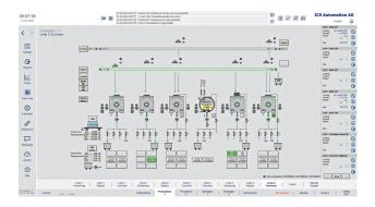
The step recipes for the desired mixing sequence and the associated parameters are now managed centrally in the higher-level process control system. On one hand, this makes it easier to implement adjustments and extensions to the recipes, and on the other hand, it enables mutual checking of the dosing and step recipes. Thanks to various analysis options, traceability and data consistency are also guaranteed.
